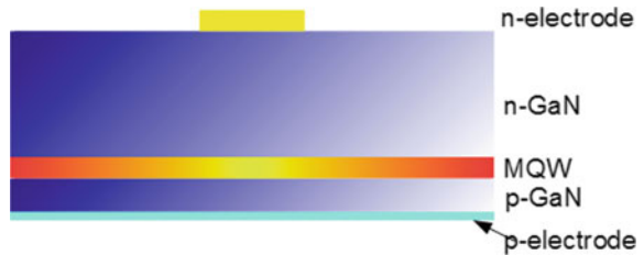
Fig. 7.20 Schematic diagram of GaN-based vertical structure LED chip
