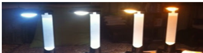
Fig. 11.1 LED lamp with dimming control to fit natural spectrum (from the left to the right are: ordinary LED, fitting daylight spectrum, the spectrum fitting incandescent lamp, candle fit spectrum)
