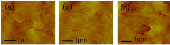
Fig. 5. AFM surface images of GaN epilayers grown on Si (111) substrates with (a) 10-pair, (b) 15-pair, and (c) 20-pair AlN/GaN SLs.
