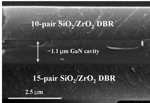
Fig. 7. Cross-sectional scanning electron microscope (SEM) image of the fabricated GaN micro-cavity structure.
