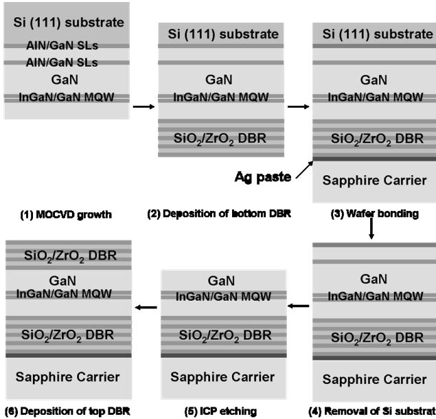
Fig. 2. Process flow chart of the GaN microcavity structure.
