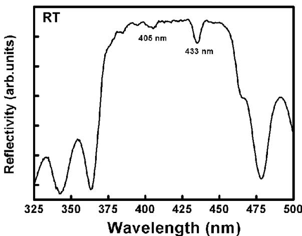
Fig. 8. Measured reflectivity spectrum of the fabricated microcavity structure.
