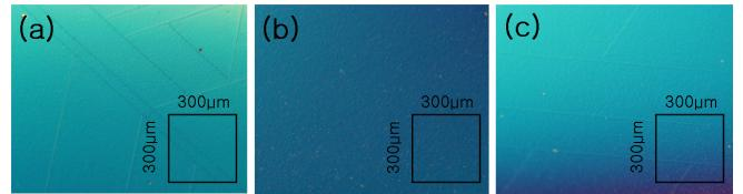
Fig. 4. Optical microscope images of the surfaces of GaN epilayer on Si (111) substrates with (a) 10-pair, (b) 15-pair, and (c) 20-pair AlN/GaN SLs.
