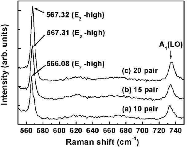
Fig. 3. Raman spectra for GaN epilayers grown on Si (111) substrates with (a) 10-pair, (b) 15-pair, and (c) 20-pair AlN/GaN SLs.
