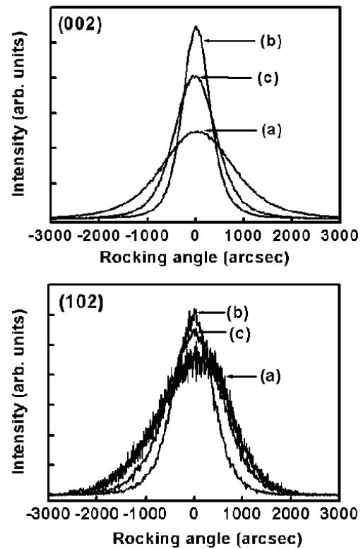
Fig. 6. HRXRD rocking curves of GaN epilayers grown on Si (111) substrates with (a) 10-pair, (b) 15-pair, and (c) 20-pair AlN/GaN SLs: (002) symmetry plane (top), (102) asymmetry plane (bottom).
