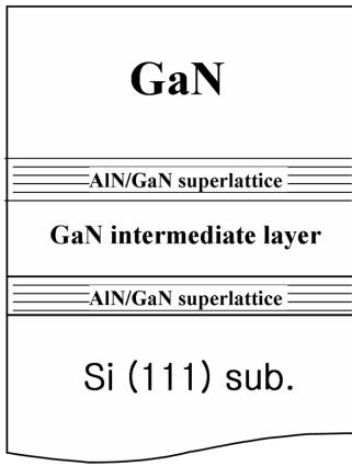
Fig. 1. Schematic cross section of the GaN epilayer grown on a Si (111) substrate.
