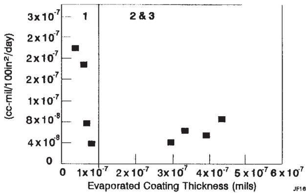
Figure 9 - Evaporated Oxygen Permeability Data
