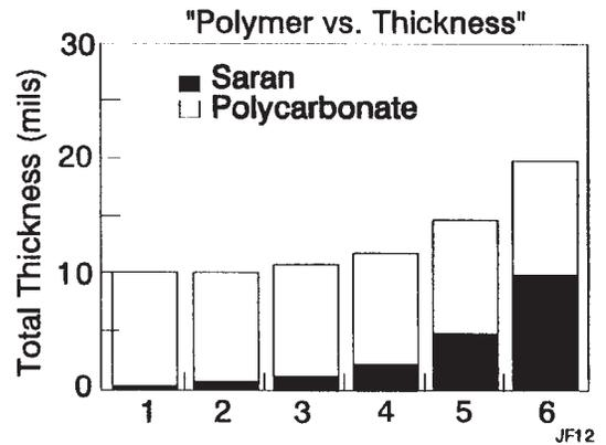
Figure 4 - Varying Polycarbonate Thickness Effects on Oxygen Transmission
