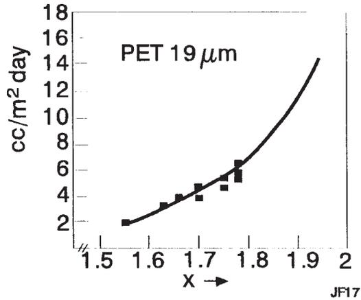
Figure 10 - Oxygen permeation vs.  $x$  of  $\text{SiO}_x$ -coated PET
