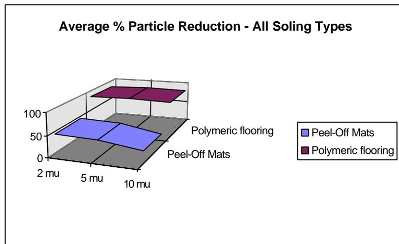
Overall, this series of tests clearly supports the view that the type of soling employed on shoes worn by cleanroom operators can have a significant effect on the efficiency of contamination control achieved at floor level, dependent on the type of control system used.
