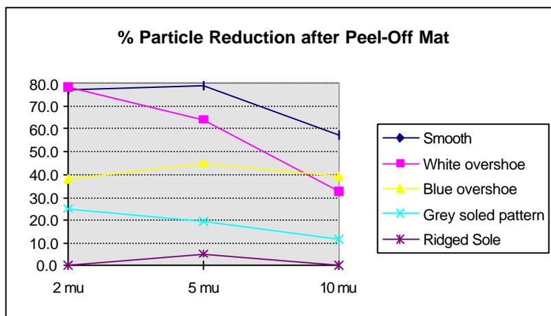
A comparison of performance of the two systems based on the average particulate reduction for all soling types is given in the table and chart below, which are largely self explanatory.
