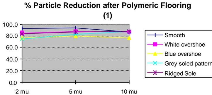
Using peel-off mats as the control surface, the highest level of particulate reduction was also obtained from the smooth soled shoe. A lower level of particulate control was achieved, however, than that with polymeric flooring. Other soling types showed extreme variability but a uniformly adverse affect on particulate removal; for the heavy ridged sole, control of particulate by peel-off mats was almost entirely ineffective. Results are illustrated in the following Table 7 and associated chart.
