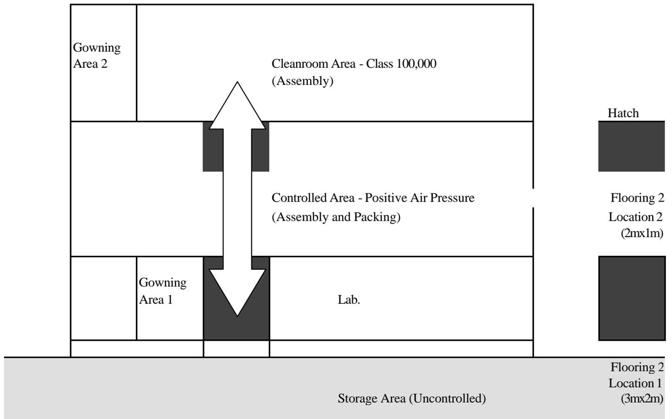
Components for assembly and packaging, together with packaging materials are drawn from the uncontrolled storage area and loaded on trolleys which pass initially into an area of controlled positive air pressure, where some assembly and all packaging operations are carried out. The majority of assembly operations are carried out in the Class 100,000 cleanroom area, where goods are accessed by means of the trolleys passing through a hatch, as shown in the diagram.
