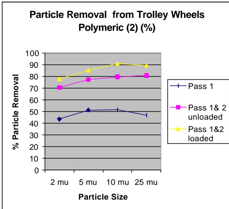
Particle counts are based on number per 10 cm<sup>2</sup> of area of wheel (about half the complete wheel area). For this area, a removal of 8 to 10,000 particles per wheel on the double pass described is obtained. This approximates to 30 to 40,000 particles per trolley, per 10 cm<sup>2</sup> of wheel area. Allowing for the actual wheel area, therefore, the number of particles removed will be approximately twice this figure at 60 to 80,000.
