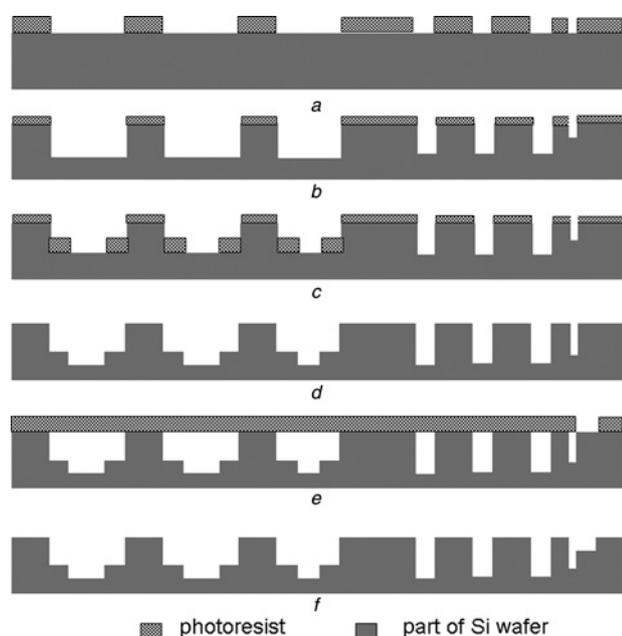
**Figure 1** Schematic of multilayer multidimensional fabrication process
