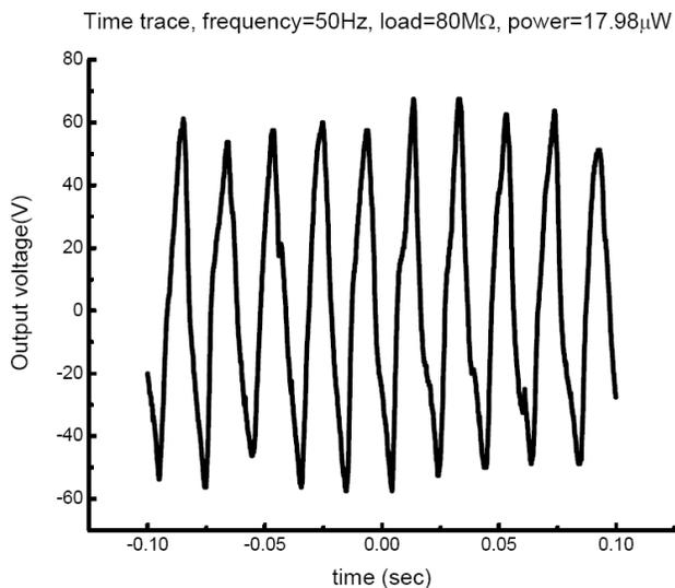
Figure 11. Output voltage at 50Hz with 80Mohm load.
