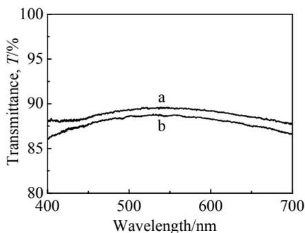
Fig.1 Transmittance of the non-coating glass substrate (a) and the WO<sub>3</sub>-Polymer coating (b) before light exposure
