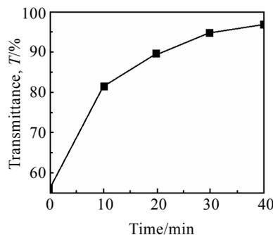
Fig.3 Decoloration transmittance of the WO<sub>3</sub>-Polymer coating irradiated at 700 nm by 60 W mercury lamps for 45 min
