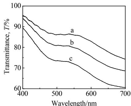
Fig.2 Transmittance of the WO<sub>3</sub>-polymer coating irradiated by 60 W mercury lamps for 10 min (a), 20 min (b), and 30 min (c)
