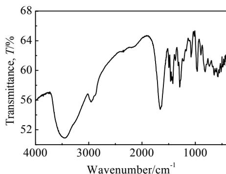
Fig.7 Transmittance of the  $\text{WO}_3$ -Polymer hybrid xerogel heat-treated at 100 °C for 60 min
