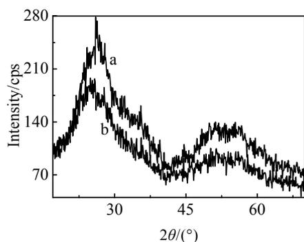
Fig.6 X-ray diffraction patterns of the  $\text{WO}_3$ -polymer xerogel heat-treated at 165 °C (a) and 80 °C (b)
