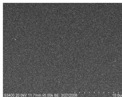
Fig.4 SEM image of the WO<sub>3</sub>-polymer coating before irradiation
