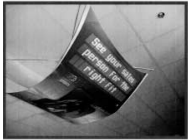
Fig. 5 Photograph of first commercial display with electrophoretic ink by E-ink's Immedia Technology in J.C. Penney stores
