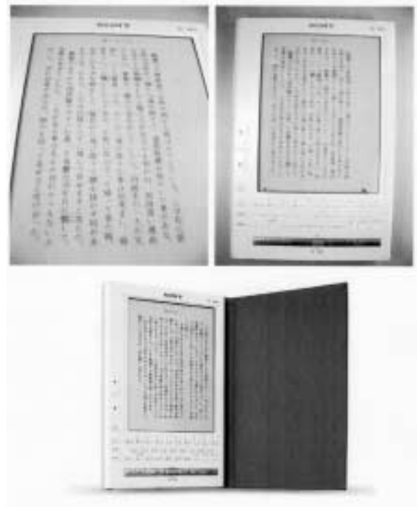
Fig. 6 Photograph of Sony Corporation LIBRIé that uses the electrophoretic ink technology of E-ink Corporation
