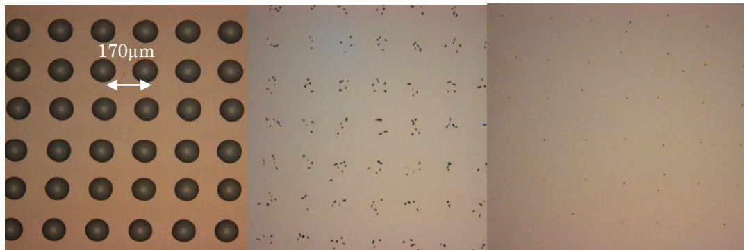
Figure 15 Inkjet printing glass substrate. To the left directly after printing. In the middle high concentrations of spacers. To the right low concentration of spacers.
