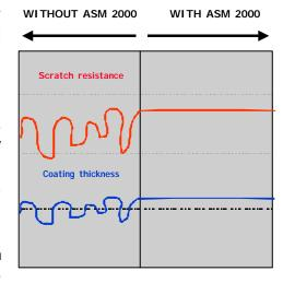
The built-in ASM 2000 in line controler eliminates all need for operator's intervention on the coating tanks
